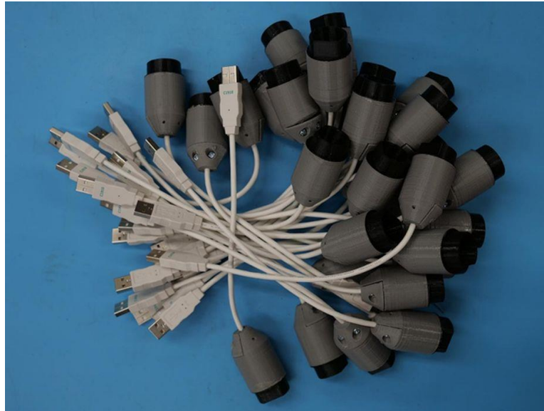
Hand-assembled 3D printed PAPR hose adapters [Source: SBU News ]
