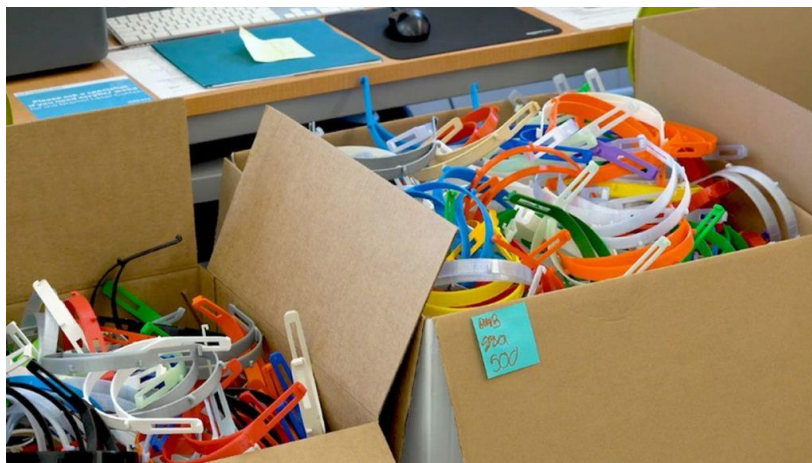
3D printed face shield components that were mass produced in the iCREATE Lab [Source: SBU Libraries ]
